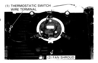
Remove the fan blade nut and washer. Remove the cooling fan from the motor shaft.
