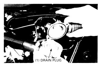
Drain the coolant from the engine; remove the drain bolt at the water pump cover and cylinder heads.
