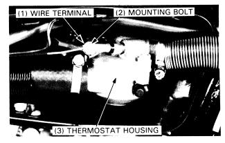
Remove the thermostat from the housing. Make sure that the O-ring is not damaged or deteriorated.
