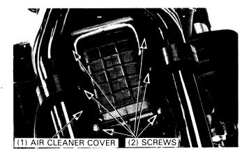
Disconnect the breather tube from the air cleaner. Remove the following:
