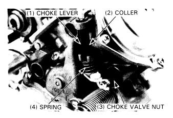
Check the choke valve and spring for nicks, grooves or other damage.
