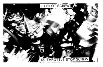
12. Drive new pilot screw plugs into the pilot screw bores with a 7 mm valve guide driver, P/N 07942-8230000. When fully seated the plug surfaces will be recessed 1 mm.
